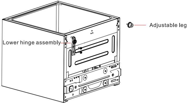
6) Put the door on lower hinge vertically, and validate the gas tightness of door gasket, then install the upper hinge by fitting screws and the hinge cover, finally cover the hole caps on upper right side.
